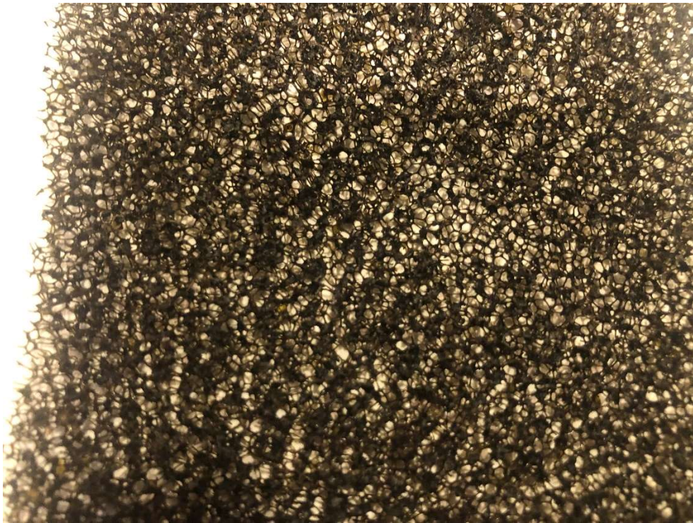
Coarse pore I-Sorbe foam sheet suitable for NPT and air sanitizing.
