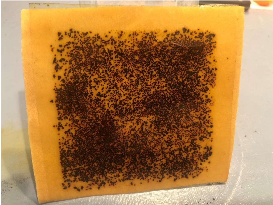
Collagen sheet adhered to an adhesive substrate covered with I-Sorbe powder.
