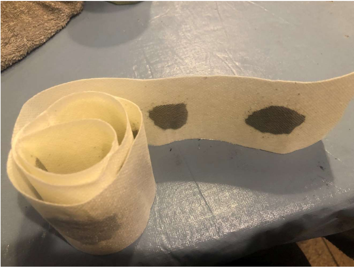
2" by 2" separate poultices, with pockets of I-Sorbe powder, on micropore covered with hydrophilic web.
