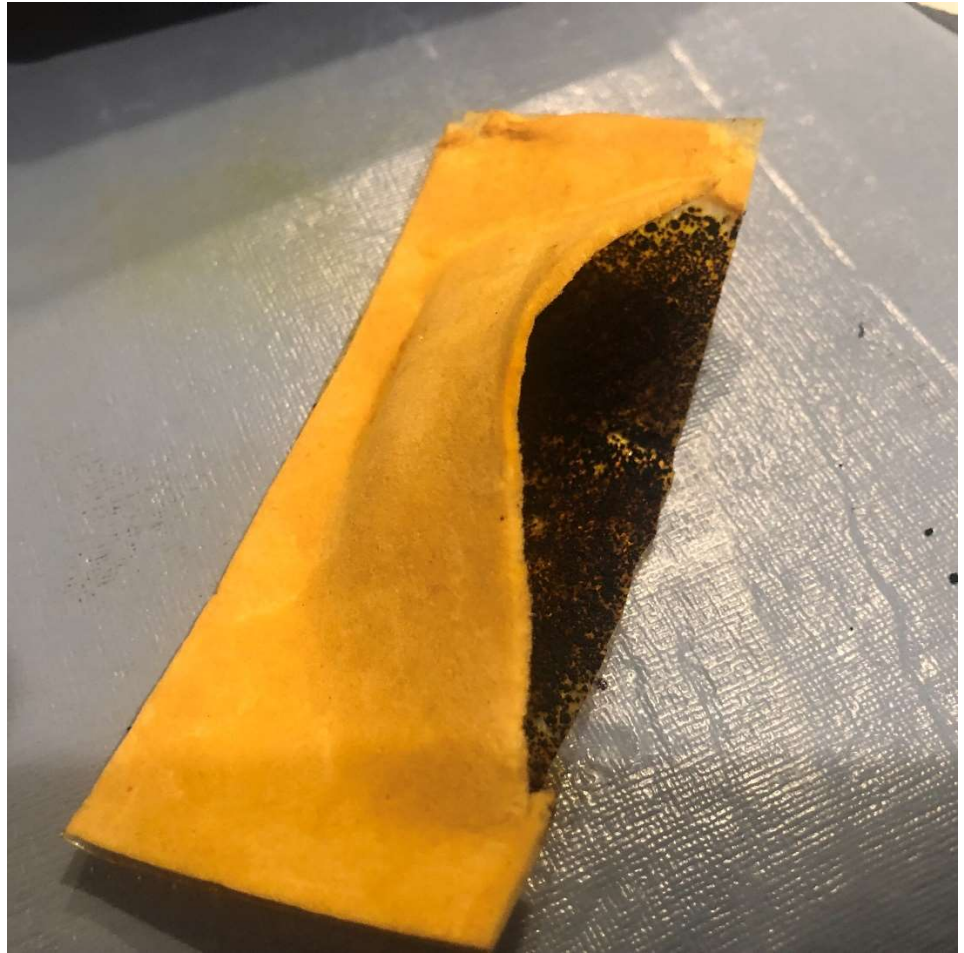
Collagen cover, fastened on powder-coated adhesive layer.
