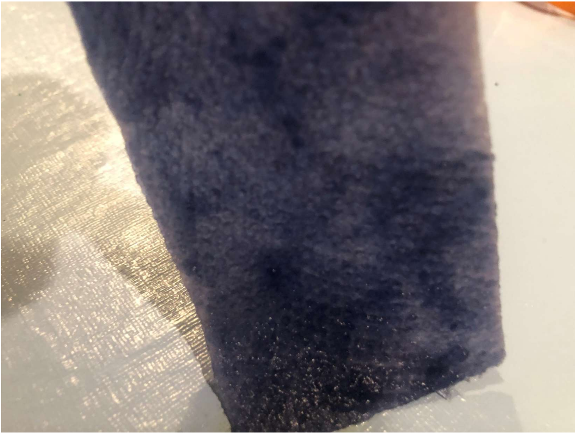
Saturated fine pore I-Sorbe foam with smooth gel surface.
