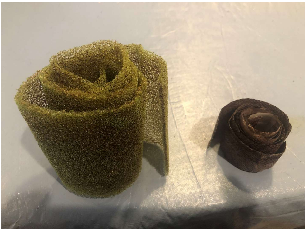
Medium pore polyurethane foam rolls suitable for a dispensing device.
