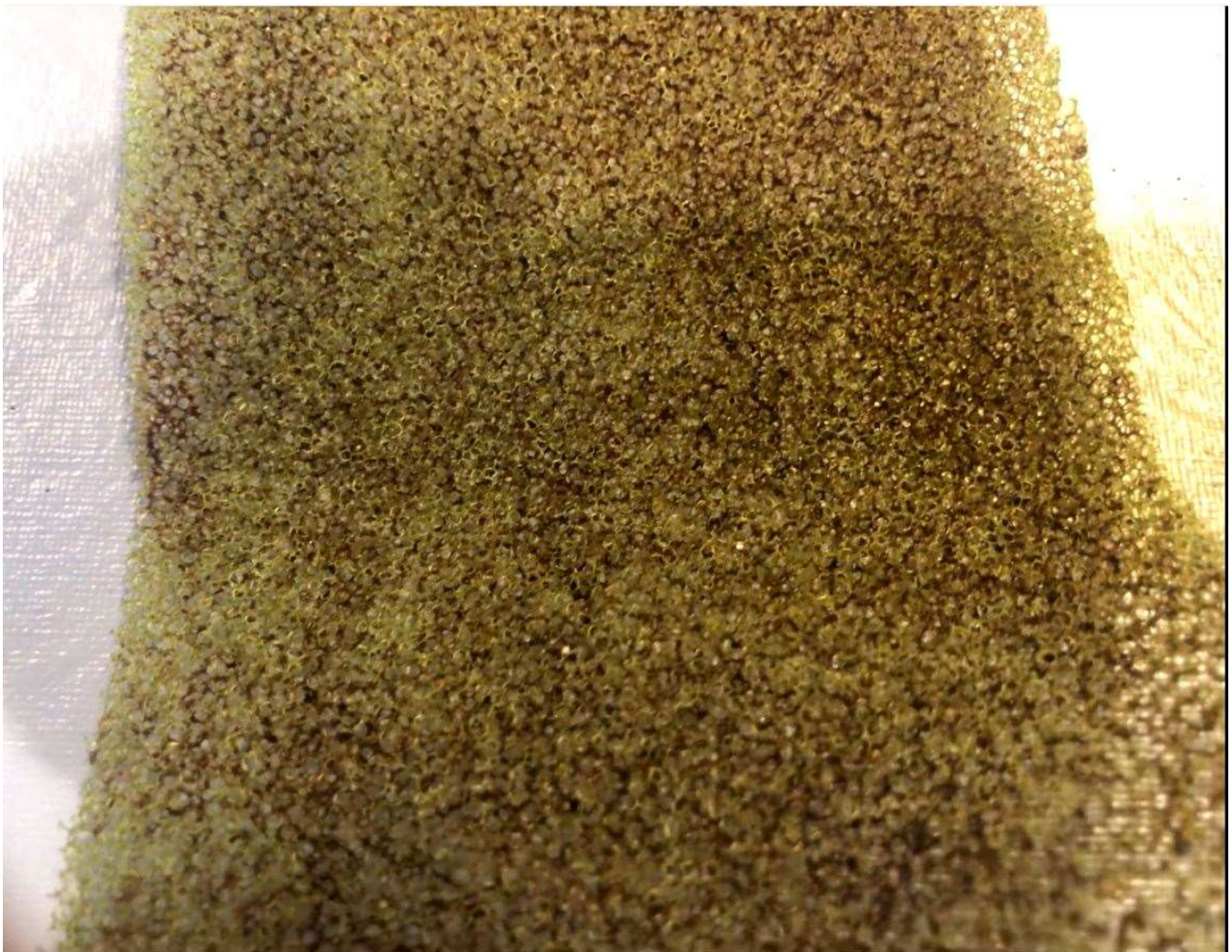
Finer poor polyurethane foam impregnated with 14% I-Sorbe powder.
